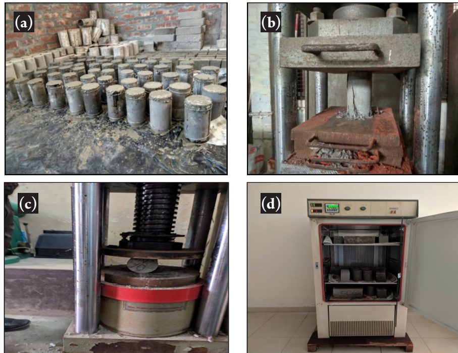
Figure 2. Sample preparation and test setup: (a) Casted concrete cylinders, (b) CS tests, (c) SPS tests, (d) Water absorption tests.
