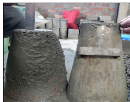
Figure 1. Slump test of concrete mix.
